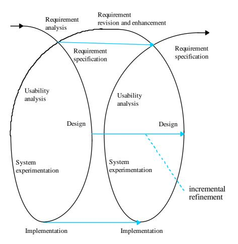
Fig. 9 Two Cycles in the Incremental Development Process
