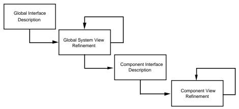
Fig. 6: The System Description Development Process
