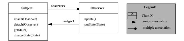
Figure 12: Simplified Structure of the Observer Pattern
