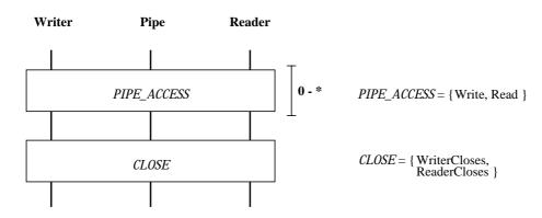
Figure 19: Pipe Interaction Architecture
