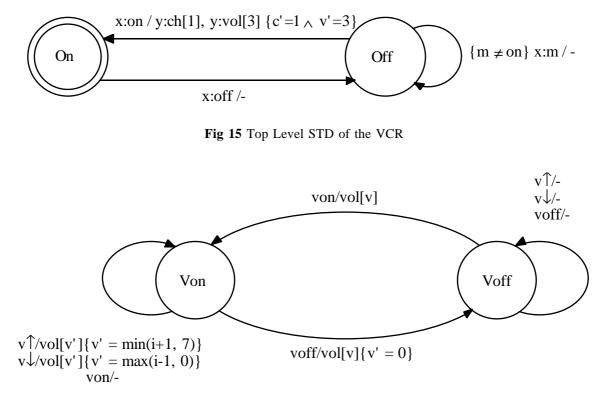
Fig. 16 STD for State Predicate Vol of the VRC
