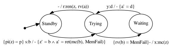
Fig. 13 STD for the Multithreaded Driver
