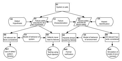
Fig. 2. A simplified example of a safety argument using GSN and context information from models
