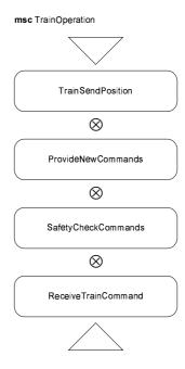
Fig. 7. TrainOperation HMSC for the BART specification
