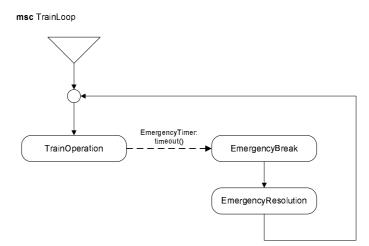
Fig. 6. TrainLoop HMSC for the BART specification
