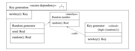
Figure 4: Key generation subsystem instance
